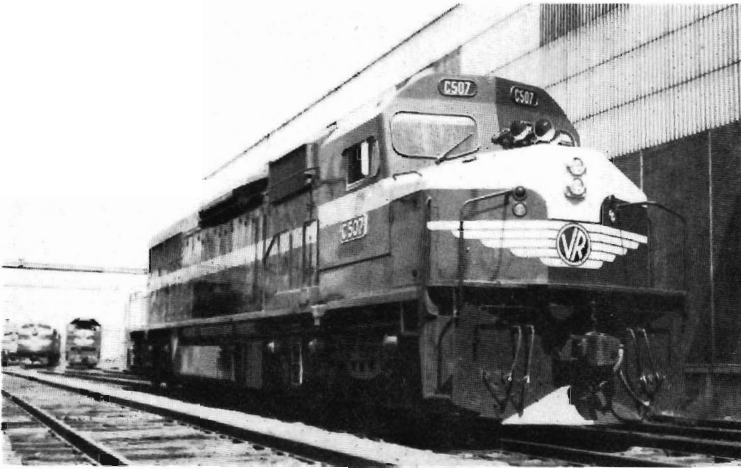
VicRail's new C-class locomotive features turbo-charging to give 50 per cent more power from a 16-cylinder engine.
