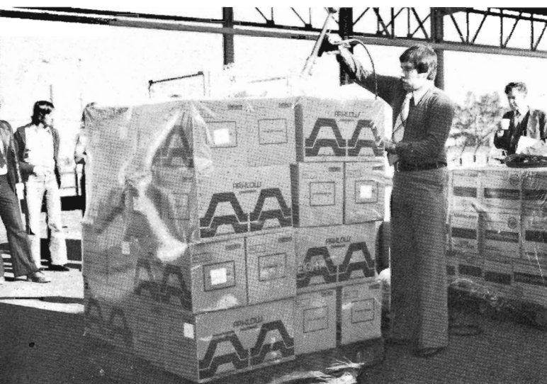
During manufacture plastic film is stretched, and after being placed around the pallet, it is heated. The film tries to shrink back to its original shape, forming a tight wrapping around the goods.
