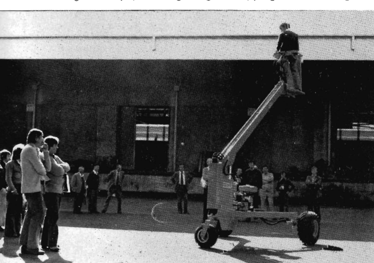
One of the popular displays was the 'Jolosapede'. This hydraulic boom ladder is operated by just one person, whose feet control the machine's direction.
